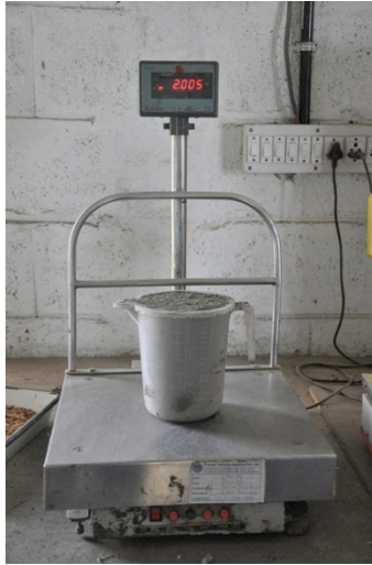
PHOTO 12. Density measurement in fresh mixture.
