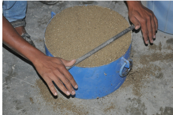
PHOTO 2. Soil prepared for loose density test with natural moisture i.e water content as found in quarry.
