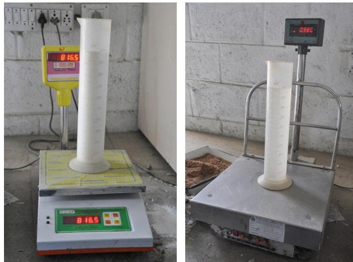
PHOTO 3. Density tests for MAXEh as well as for the water. Similar test was used for cement.
