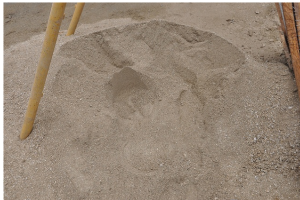
PHOTO 1. Silty sand soil obtained from Nelamangala site.
