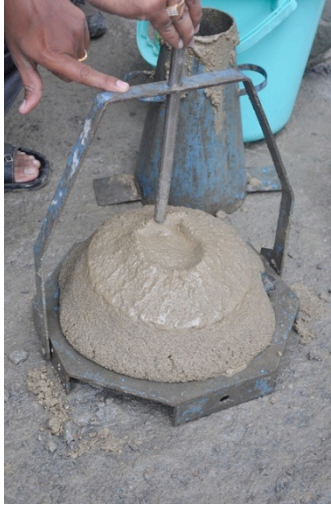
PHOTO 6. Slump test in water needed trials.
